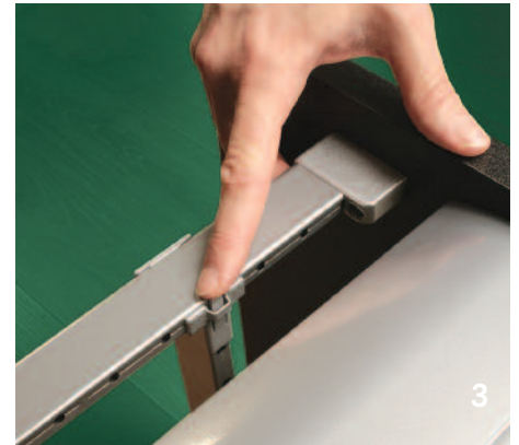
3. Dividers are moved by depressing the tabs on the end caps which index into holes underneath the side rails.
