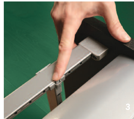
3. Dividers are moved by depressing the tabs on the end caps which index into holes underneath the side rails.
